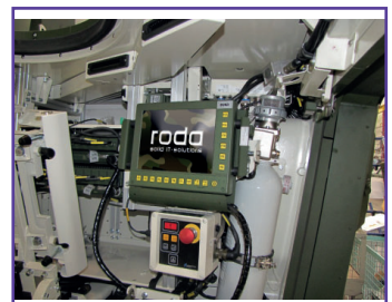
RD10-XGA vehicle installation
