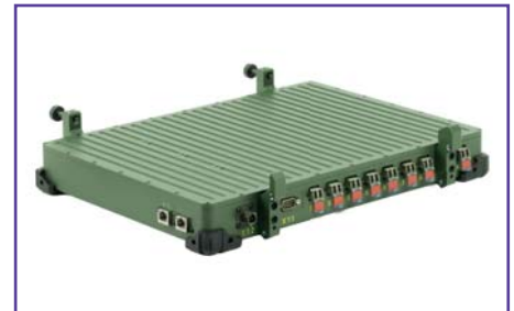
The 8-port FO switch can also be used as a stand-alone solution
