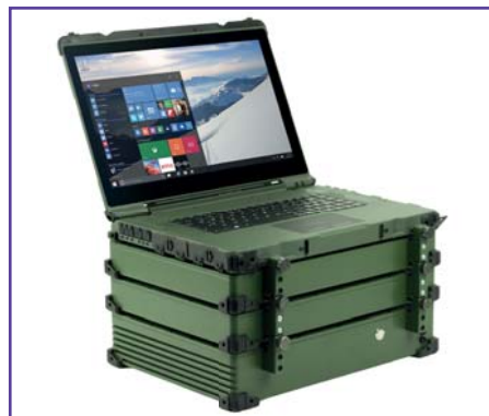
The individual RW11 mission modules are screwed on the front and positioned and secured on the back by holding bolts
